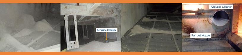
Ash buildup in coal-fired SCR reactors is a common occurrence that negatively affects gas flow and catalyst life. CORMETECH employs a combination of acoustic cleaners and ash sweepers to eliminate this industry-wide problem and offers the following features:
