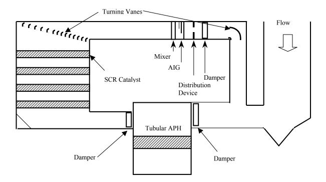
Figure 2: Ammonia Distribution at Catalyst Inlet
